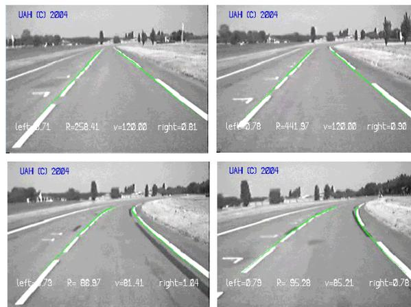
**Fig. 1.** Lane tracking example in a sequence of images. The green lines represent the estimated lines of the road. The example also depicts the error between the left wheel of the car the the left lane (left), the error between the right wheel of the car and the right lane (right), the radius of curvature of the road estimated at a lookahead distance of 50m (R), and the maximum recommended velocity to bend the curve (V) according to the radius of curvature.
