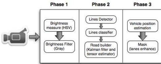
Figure 1. Algorithm architecture.
