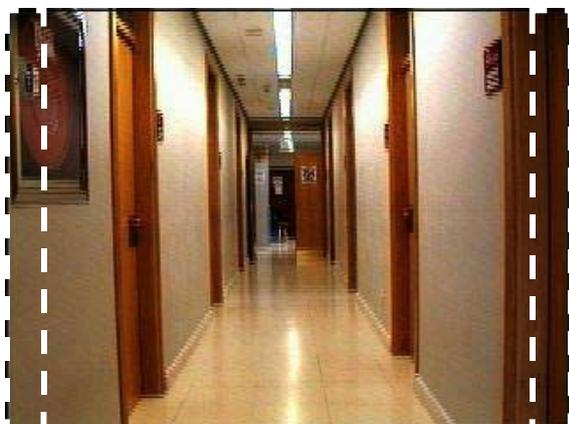
Fig. 2. Lateral windows to extract door frames and predict immediate state transitions with "Follow Corridor" action.
