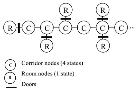
Fig. 5. Topological model of figure 2 environment.
