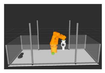
Fig. 1. Robot Model: the robot model and its working environment are shown. There are two different objects placed in the working scene: a can (cylinder) and a ball (sphere), which is depicted with a safety area around it
