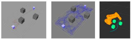
Fig. 3. In this figure the differences between probabilistic road-map and tree-based planning strategies are shown using KPIECE (left image) and PRM planner (center image). They are employed on an environment close to the real cases they will be faced. These
