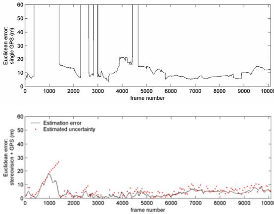
**Fig. 4.** Euclidean distance error ( $\epsilon = \sqrt{X^2 + Z^2}$ ) using standard single GPS (up) and our combined SLAM system (down). Global covariances uncertainties for each node are shown as well.
