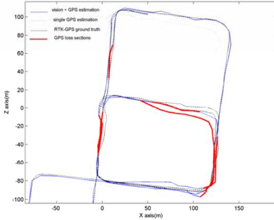
**Fig. 3.** Path estimation using only a standard low-cost GPS (dotted line), our SLAM method by means of vision and GPS (solid line), and the ground truth (dashed line). Thick red lines indicate path sections where GPS was unavailable.
