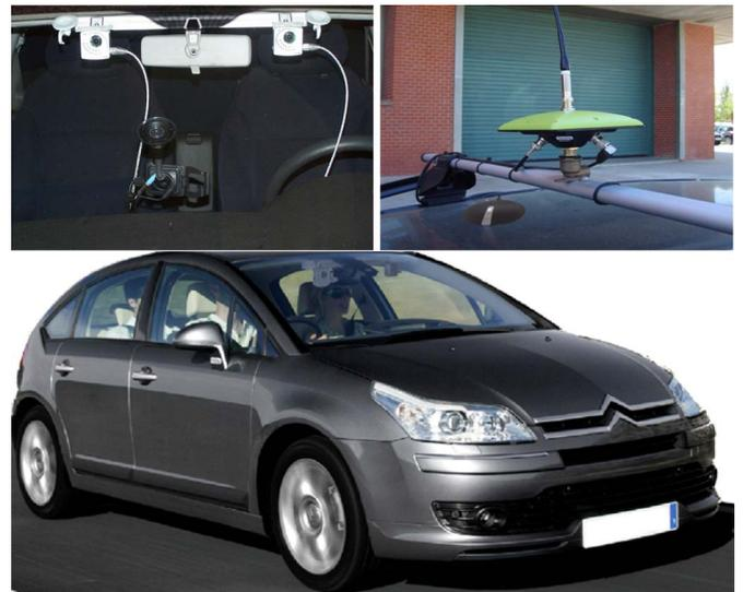
Fig. 2. (Bottom) System architecture mounted on a commercial car. (Top left) Stereo-vision system and low-cost GPS. (Top right) Ground truth RTK-GPS.
