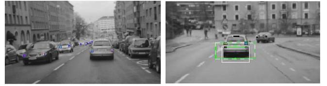
(a) Detected lights in a frame (b) Gating of measurements
