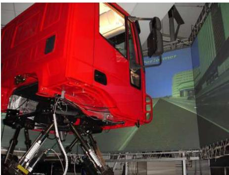
Fig. 1. Real truck cab simulator
