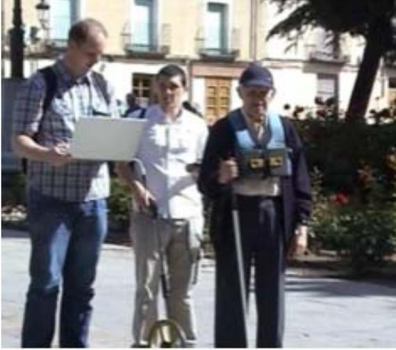
Fig. 8. The stereo camera system is attached to chest of the visually impaired user by means of a non-invasive orthopedic vest. Then the camera is connected to a small laptop by means of a firewire cable.
