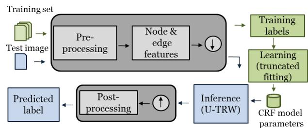
Fig. 1: Overall system workflow. Down and up arrows correspond with the downsample and upsample performing with superpixels.
