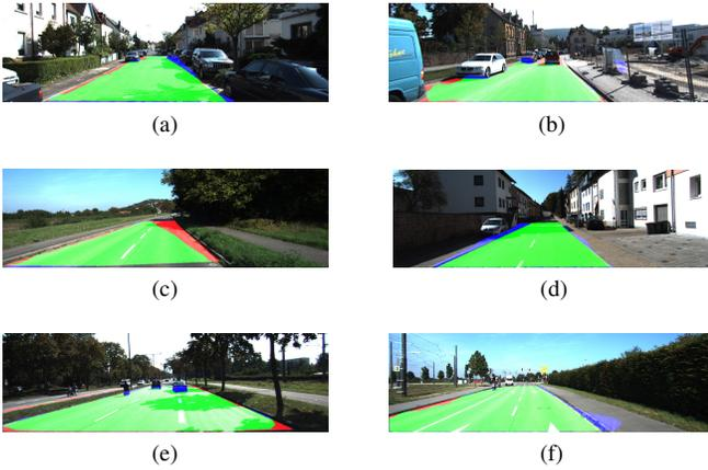
Fig. 6: Examples of road detection images for the test set obtained from the public benchmark suite, red denotes false negatives, blue areas correspond to false positives and green represents true positives (a),(b) UU; (c),(d) UM; (e),(f) UMM
