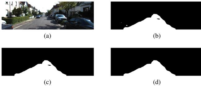
Fig. 5: Post-processing of a sample result from the pixelwise road inference: (a) input image (b) predicted pixel labels (c) removal of false positives using a morphological opening (d) removal of false negatives using a morphological closing.
