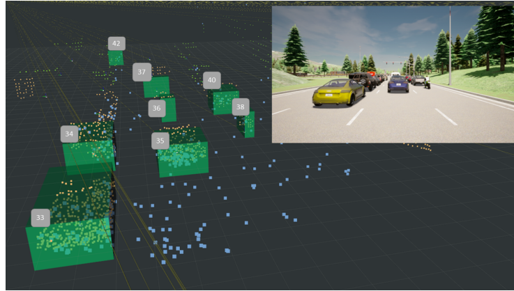
Fig. 1: Performance of the DAMOT method in a Traffic Jam use case in AD PerDevKit dataset. Tracked objects are shown as green Bounding Boxes.
