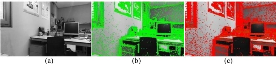
**Fig. 6** Experimental validation of the IMU/LSD-SLAM algorithm (a) level gray image, (b) Features extraction and depth estimation, (c) Colour representation of the estimated depth variance.
