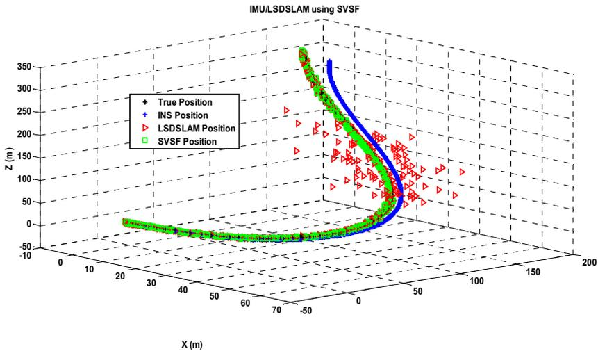
**Fig. 3** Comparison of IMU, LSDVSLAM and SVSF position when visual information is not available
