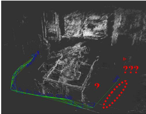
**Fig. 11** Pose estimation and 3D map construction using LSD-SLAM (dashed ellipse images missing, LSD-SLAM cannot estimate any Bebop position).
