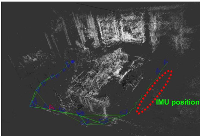
Fig. 14 Pose estimation and 3D map construction using IMU/LSD-SLAM (dashed ellipse visual information is not available, IMU/LSD-SLAM can estimate the Bebop position)
