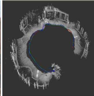
**Fig. 9** Localization and 3D map building using MAV-SLAM algorithm
