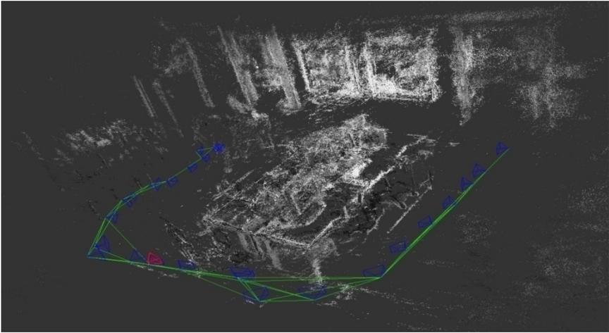
**Fig. 7** Bebop localization and 3D map building using IMU/LSD-SLAM
