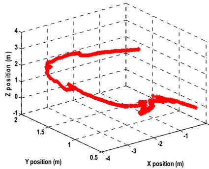
Fig. 13 Bebop position given by the IMU
