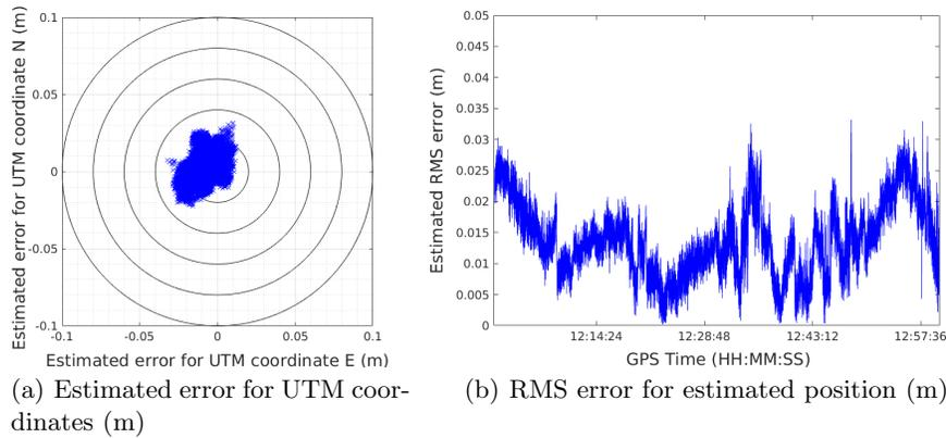
**Fig. 5.** GPS+GLONASS performance for differential receiver with Fixed-RTK
