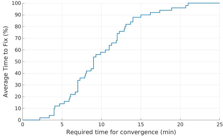
**Fig. 6.** Convergence time for RTK-Fixed solution.
