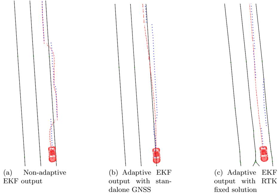
**Fig. 12.** Adaptive EKF Robustness Example
