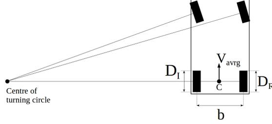
**Fig. 7.** Vehicle diagram - Ackerman steering geometry
