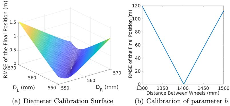
Fig. 8. Odometry Calibration
