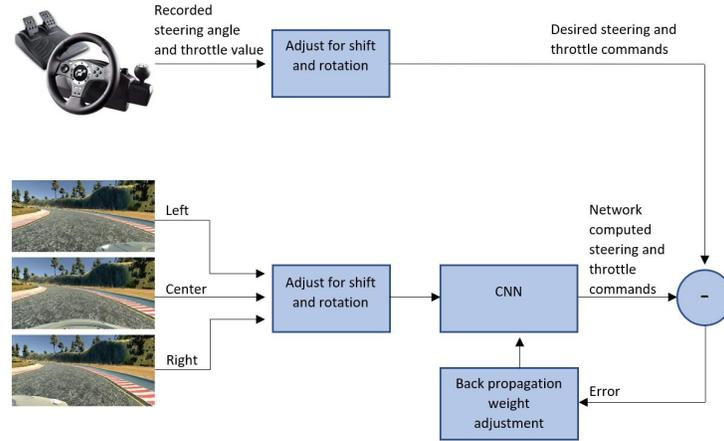
**Fig. 1.** Left, center and right images from driving simulator captured to train CNNs
