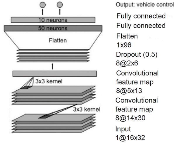
Fig. 2. TinyPilotNet architecture
