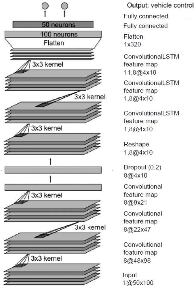
Fig. 4. DeepestLSTM-TinyPilotNet architecture
