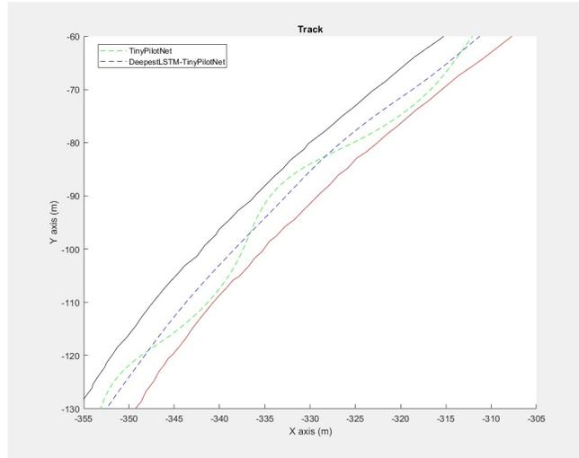
**Fig. 12.** Fragment of track showing TinyPilotNet and DeepestLSTM\_TinyPilotNet car trajectories.
