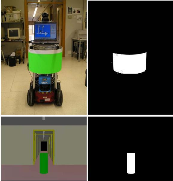
Fig. 4. Robots detection in real environment and simulation.
