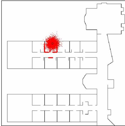
Fig. 12. Initial gaussian belief for robot 2 ( $\sigma = 0.8$ ).
