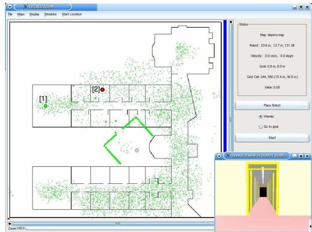
Fig. 11. Initial uniform belief's robot.
