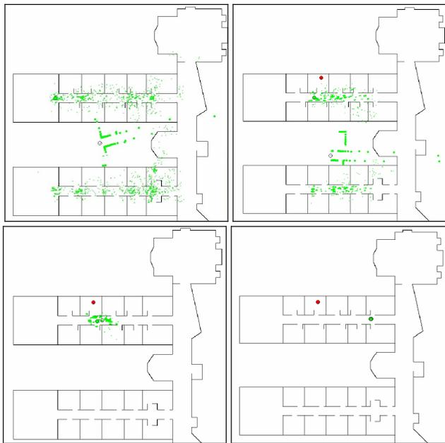
Fig. 13. Belief's robot 1 (Robot 2 with gaussian belief with  $\sigma = 0.8$ ).
