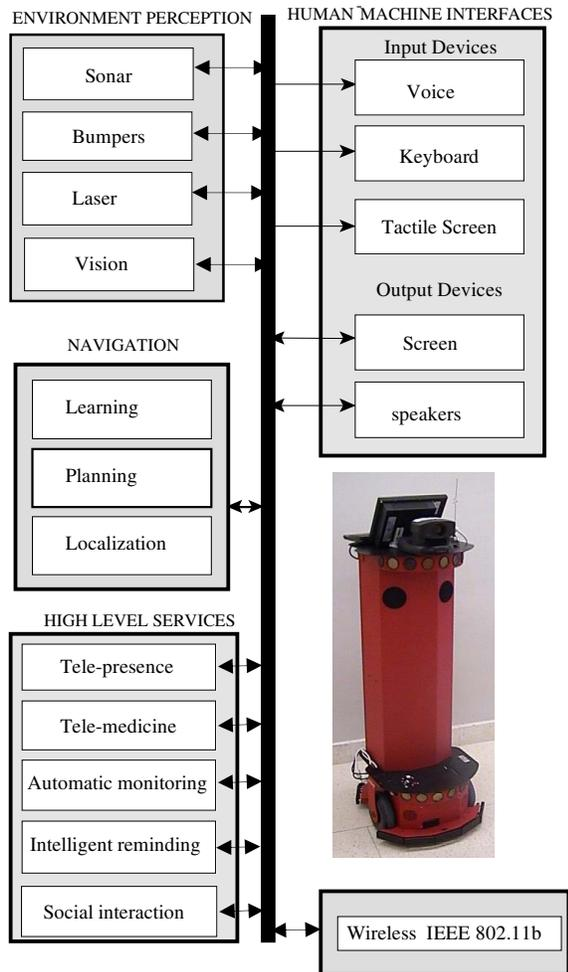
Fig. 2. General architecture of the robots.
