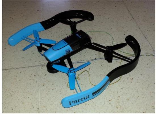
Fig. 1. Bebop Drone from Parrot, the commercial drone used as flying unit in our experiments.
