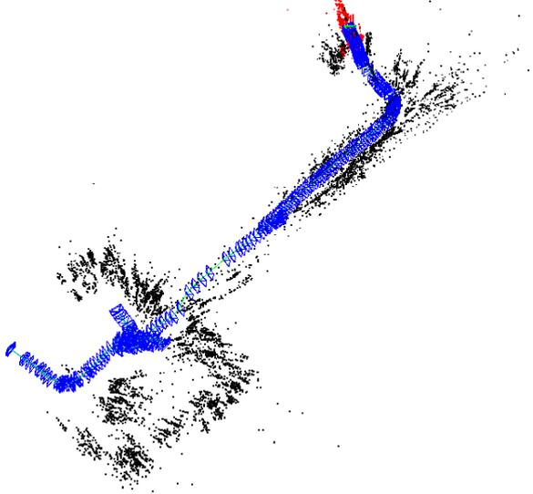
Fig. 4. Results of ORB-SLAM estimating the pose of the camera in the same environment of Fig. 3.
