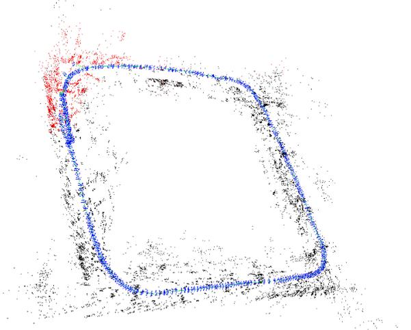
Fig. 5. Results of ORB-SLAM estimating the pose of the camera around a square.
