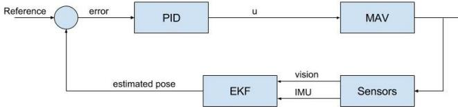
Fig. 6. PID Controller Blocks Diagram
