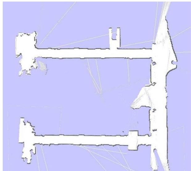
Fig. 5. Global map using scan-matching.
