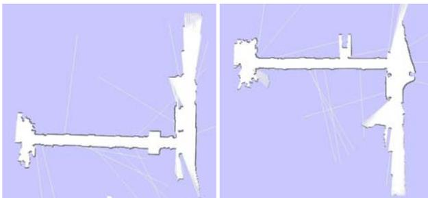
Fig. 4. Partial maps built by robots.
