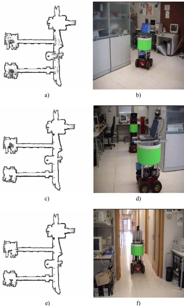
Fig. 7. Collaborative multi-robot Monte Carlo localization.
