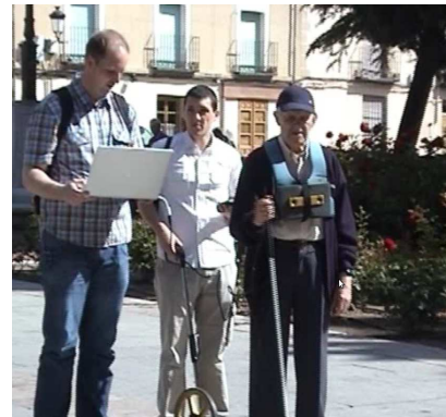
Fig. 6. The stereo camera system is attached to chest of the visually impaired user by means of a non-invasive orthopedic vest. Then the camera is connected to a small laptop by means of a fireware cable.
